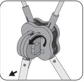
Loosen knob on rear of Body to adjust back leg out and into supporting position.
