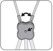
Press button on body and hold to release gear mechanism. Begin moving top arms with hooks away from each other. Release button.
