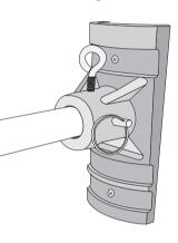
Insert the pole into the holder on the bracket. Line the hole on the end of the pole with the
