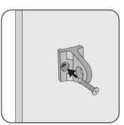
Insert screw into holes found on each side of the D-bracket and drill into wall (mounting screws are not included).
