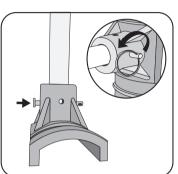
Insert the pin through the bracket and the pole. Attach the ring to the hole on pin.
