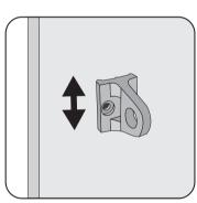
Position the bottom D-bracket against the wall.
