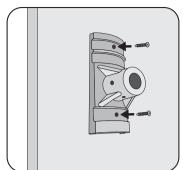
Insert screw into holes found at the top and bottom of the pole mount and drill into wall (mounting screws are not included).
