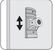
Determine the desired height of the wall bracket. Position the top bracket with the tapered end pointing up.
