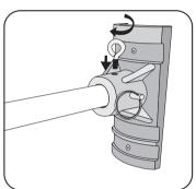
Hand tighten the eye bolt in the threaded hole until secure. (Repeat steps 1 to 3 for multiple poles and brackets).
