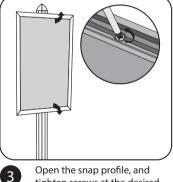
Open the snap profile, and tighten screws at the desired height.
