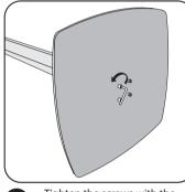
Tighten the screws with the 2 allen wrench provided.
